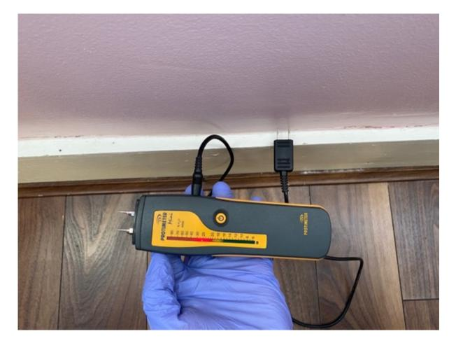
A red reading on the Protimeter confirms that the percentage level of moisture within the wall is at the higher end of the spectrum and in this case, I suspect the damp penetration is a result of the bridging of the damp proof course.
