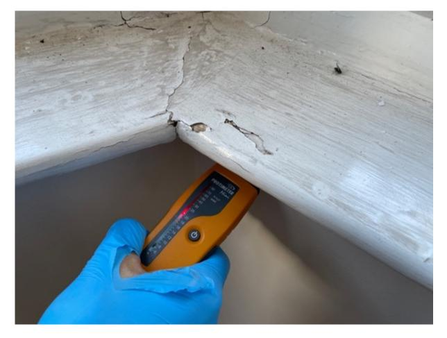
Protimeter tests were undertaken throughout the property, and I was able to obtain red readings throughout, which all would be due to the aforementioned defects, such as the failed external sills, rendering, failed roof coverings and also the insufficient number of radiators throughout the property, which are not fit for purpose and are too small in size, relevant to the rooms.
