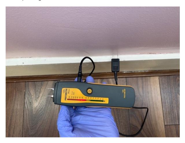
A red reading on the Protimeter confirms that the percentage level of moisture within the wall is at the higher end of the spectrum and in this case, I suspect the damp penetration is a result of the bridging of the damp proof course.
