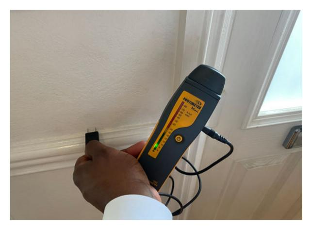
Damp meter tests were taken to the perimeter of the property and walls throughout, at low, mid and high level. All readings returned with a green reading, which is effectively a dry damp meter reading, and the result we would look for as surveyors.
